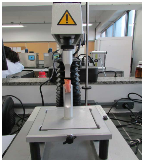
Figura10. (a) Probe Warner-Bratzler (b) Probe Volodkevich Bite Jaws.
