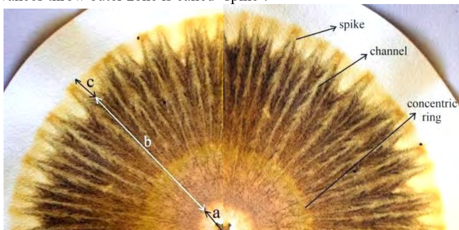
Figure 7. Zones and forms of soil chroma: central zone (a), inner zone (b) and outer zone (c), channels, concentric rings and spikes.
