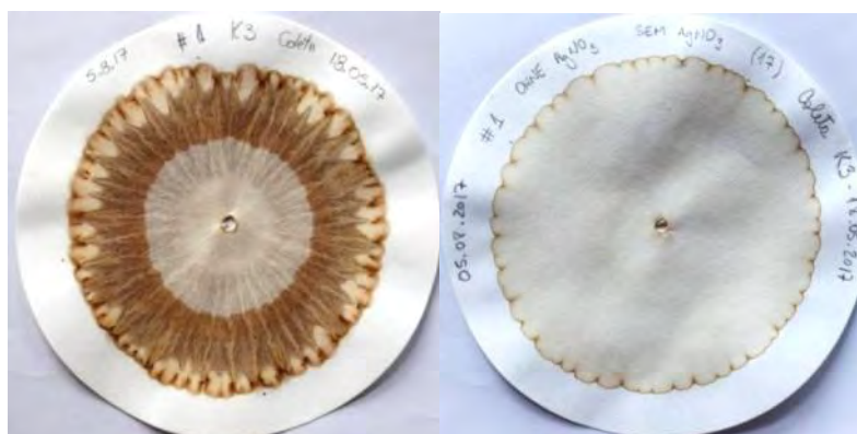
Figure 3. \text{AgNO}_3 effect on chromatography. The same compost sample reacted with NaOH and run on \text{AgNO}_3 -sensitized filter paper (left) and non-sensitized filter paper (right).
