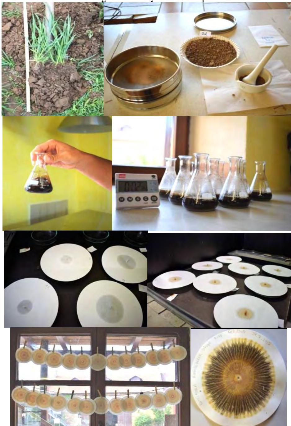
Figure 1. Chromatography process for soil: a) collection in field; B) drying, maceration and sieving; C) mixing 5 g of soil with NaOH and stirring; D) rest for 6 hours; E) impregnation of circular filter paper with AgNO 3 ; F) running the soil solution on impregnated paper; G) drying in indirect light; H) final image.
